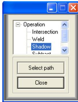
From Operation screen, selects **Welding/Shadow**, then click **Select path**. With the help of the mouse, click on the object that you want to create a shadow. WinPCSIGN will automatically open shadow configuration screen. Select the direction, color; and the shadow thickness (X and Y values). You can also add inside shadows.
