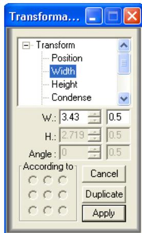
Select the element to modify. From Transformation bar select **Width**, enter the desired value **W** and click Apply.
