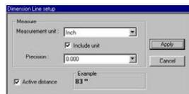
This window will enable you to configure which measurement unit is used, whether to include the unit or not, it is also used to determine the precision used.
